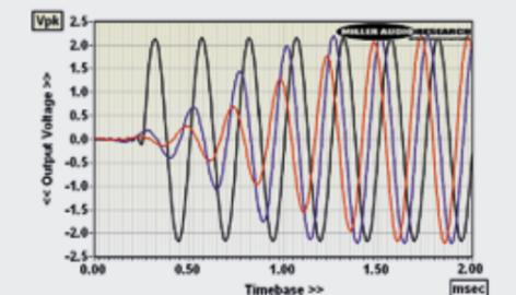
**ABOVE: 4kHz toneburst (bypass, black trace) showing attenuation and latency with minimum 'Repair 1' (blue trace) versus maximum 'Repair 10' (red trace)**
