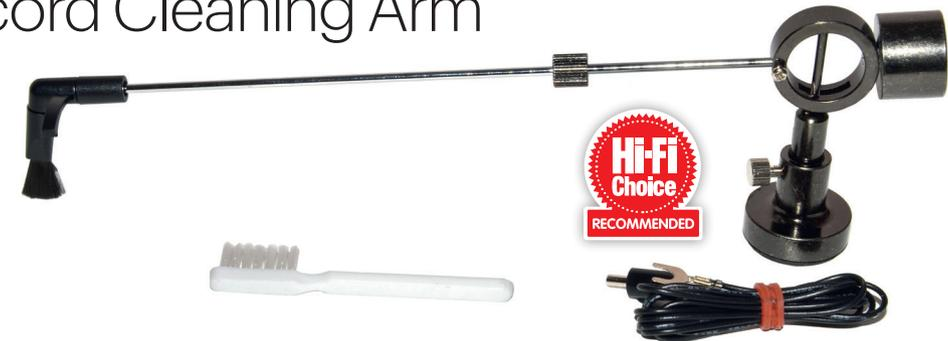
A particular feature of this device is the small earth wire that at one end plugs into the base of the unit and at the other is fastened to the earth tag of your turntable deck or phono amplifier to dissipate the static charges from the tip of the carbon fibre brush away to earth. Although the base is fitted with an adhesive pad to fix it to the record player, I find that the weight of the base alone is sufficient to hold it in place. I initially find that the brush gets stuck in the
