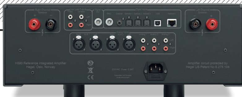
ABOVE: Top left of the rear panel are fixed and variable preamp outputs, with five line inputs (two balanced on XLRs, three single-ended on RCAs). The row of digital ins includes three optical, two coaxial (RCA/BNC), a USB Type B and an Ethernet port
