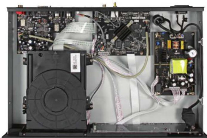
As with other Arcam products, the CDS27 is neatly-constructed both inside and out. Note how the unscreened switch-mode power supply (right), analogue board (top left) and digital board (top centre) are separated from each other to reduce noise problems. The disc transport is also clearly visible.
