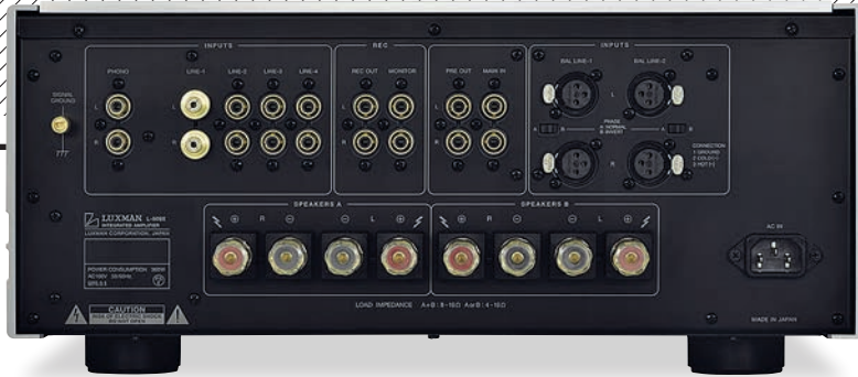
ABOVE: No digital or network connections here: just MM/MC phono, four line-ins on RCAs and two sets of XLRs, plus a good old-fashioned tape loop and pre-out/power amp inputs, with internal connection broken by front-panel 'separate' button
