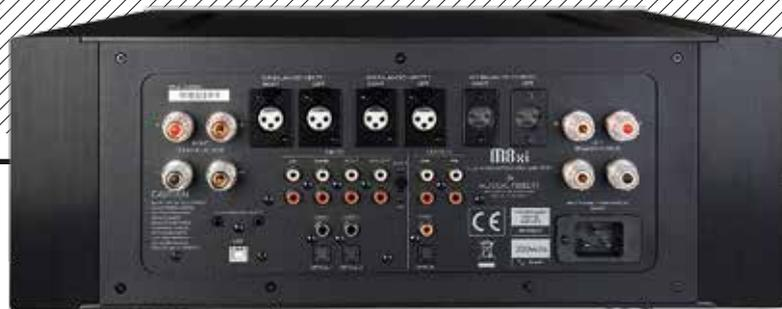
**ABOVE:** Five line ins (three on RCA, two balanced on XLRs), USB-B and pairs of coax/optical digital ins are joined by balanced and single-ended pre outs (XLR/RCA), one fixed line out (RCA) and coax/optical digital outs. There are two sets of floating (live negative and positive) 4mm speaker outlets per channel for easy bi-wiring
