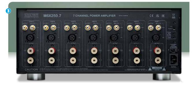
3. Generous chassis dimensions result in a well-spaced rear panel with XLR/RCA in and gold-plated speaker terminals
