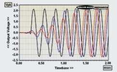
ABOVE: 4kHz toneburst (bypass, black trace) showing attenuation and latency with minimum 'Repair 1' (blue trace) versus maximum 'Repair 10' (red trace)
