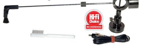
A particular feature of this device is the small earth wire that at one end plugs into the base of the unit and at the other is fastened to the earth tag of your turntable deck or phono amplifier to dissipate the static charges from the tip of the carbon fibre brush away to earth. Although the base is fitted with an adhesive pad to fix it to the record player, I find that the weight of the base alone is sufficient to hold it in place. I initially find that the brush gets stuck in the
